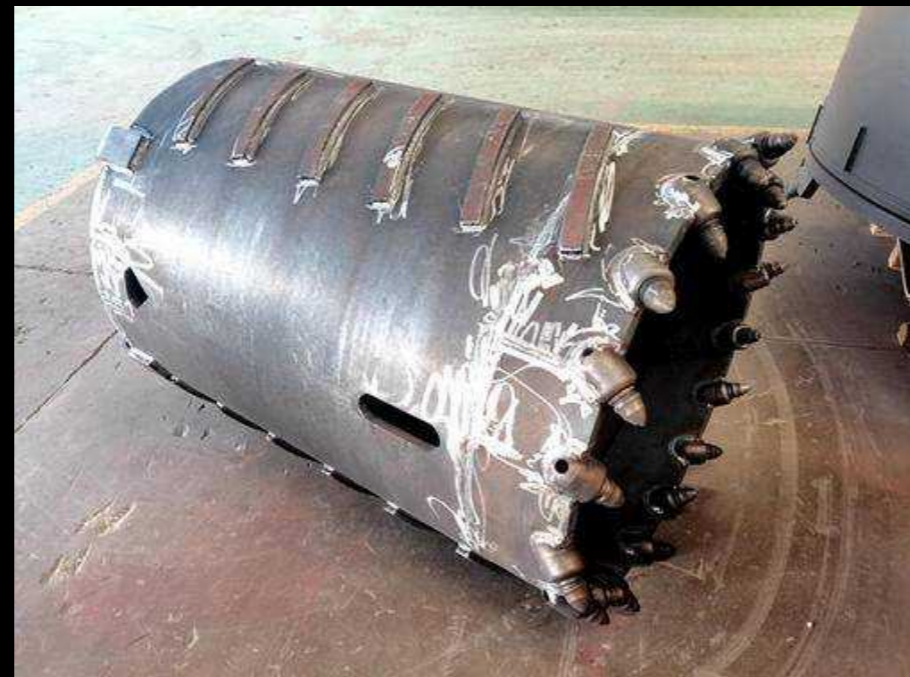
Core Barrel with Round Shank Chisel Teeth
